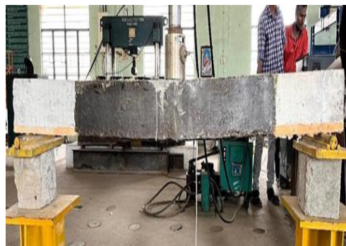
Figure 8. 50 mm ECC layered retrofitted by BFRP Sheet
