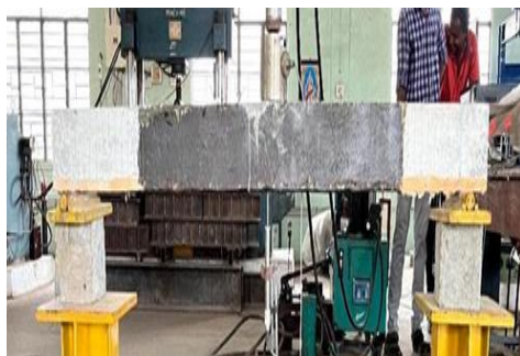
Figure 7. 20 mm ECC layered retrofitted by BFRP
