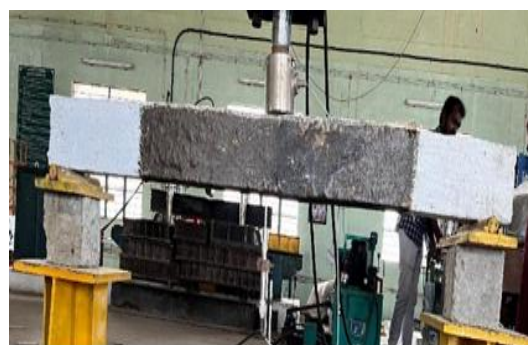
Figure 6. Control beam wrapped with BFRP sheet
