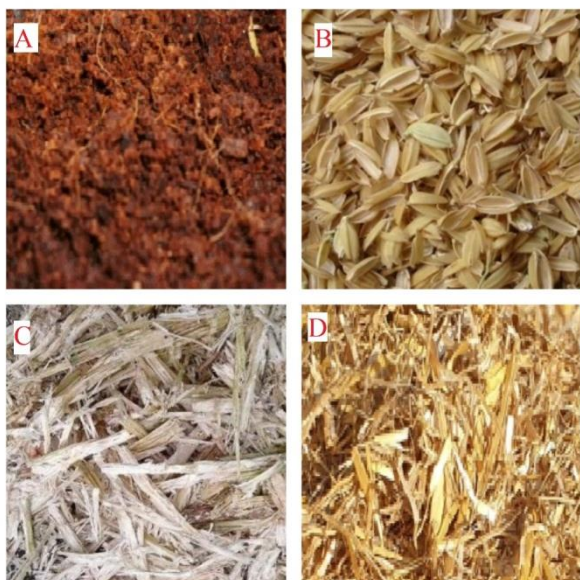
Figure 1. Agro industrial wastes. A) Coconut Coir Dust B) Rice husk C) sugar cane bagasse D) Wheat Straw
