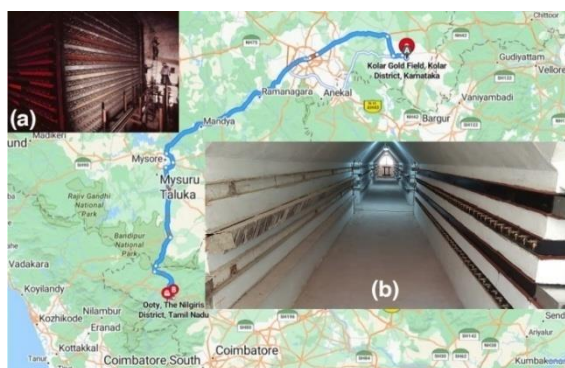
Figure 1. A view of the transportation of steel pipes by road from the underground KGF laboratory to Ooty, the current site of the GRAPES-3 experiment. Inset (a) shows the arrangement of the counters in the 2300-meter-deep underground laboratory prior to their relocation. Inset (b) shows the current condition of the counters incorporated into the newly designed large-area tracking muon telescope
