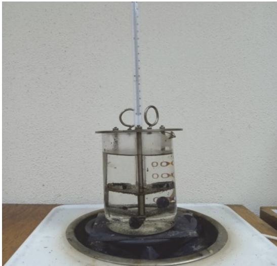
Figure 2. Determination of softening point using the "Ring and Ball" device
