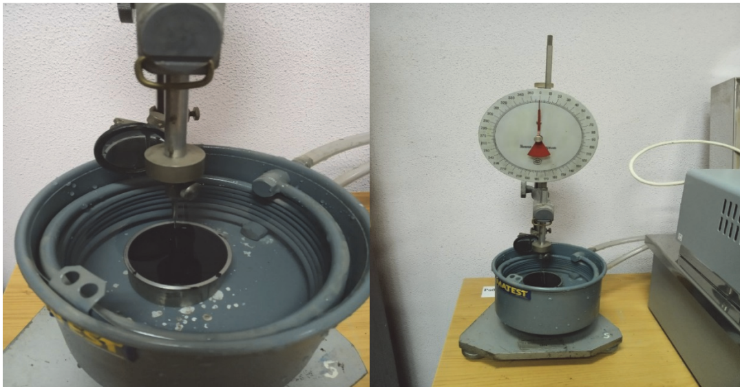
Figure 1. Determination of the penetration depth
