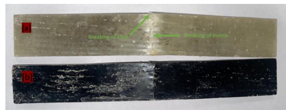
Figure 3. Photographs illustrating the damage mechanism in (a) neat epoxy composite and (b) CNT/MXN reinforced hybrid composite sample
