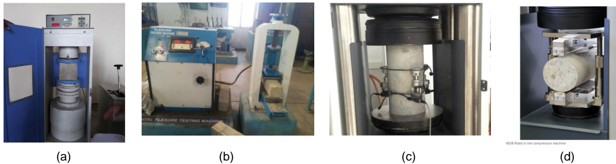
Figure 2. (a) Compressive strength test (b) Flexural strength test (c) Modulus of elasticity test (d) Split tensile strength test
