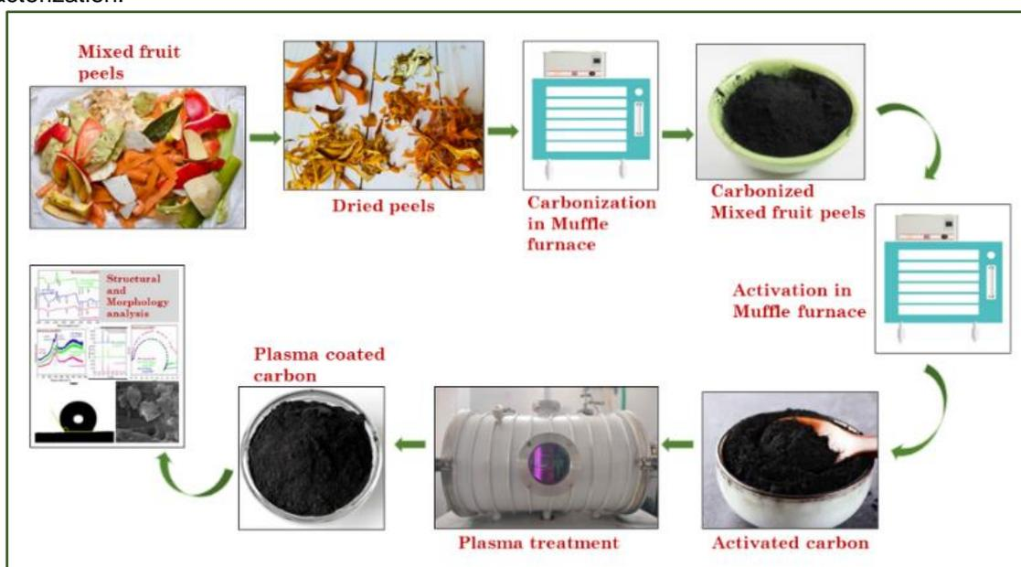
Figure 2. Synthesis of Mixed fruit peel activated carbon
