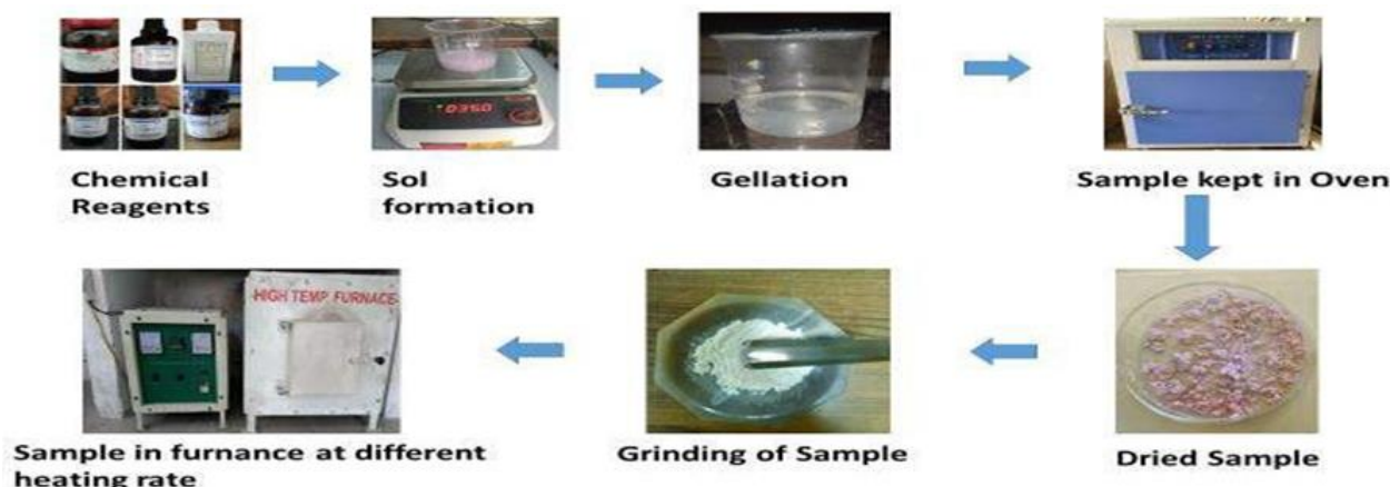
Figure 1. Experimental view of preparation of samples via sol-gel route
