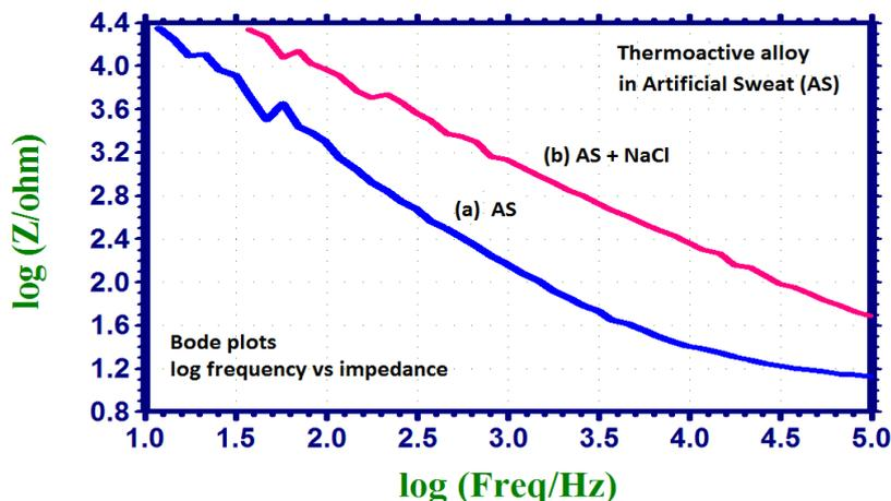
Figure 3. Bode plots (log frequency vs impedance) of Thermo active alloy immersed in various test solutions: (a) Artificial sweat (b) Artificial sweat + NaCl (100 ppm)
