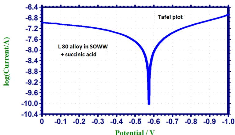
Figure 2. Polarisation curve of L 80 alloy immersed in SOWW + succinic acid
