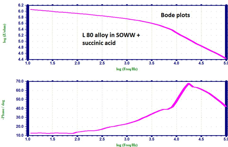
Figure 9. Bode plots of L 80 alloy immersed in SOWW + succinic acid
