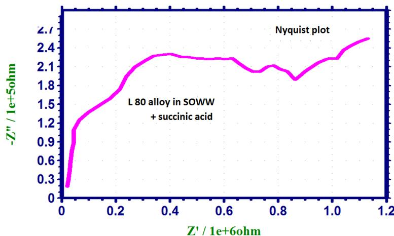
Figure 8. Nyquist plot of L 80 alloy immersed in SOWW + succinic acid
