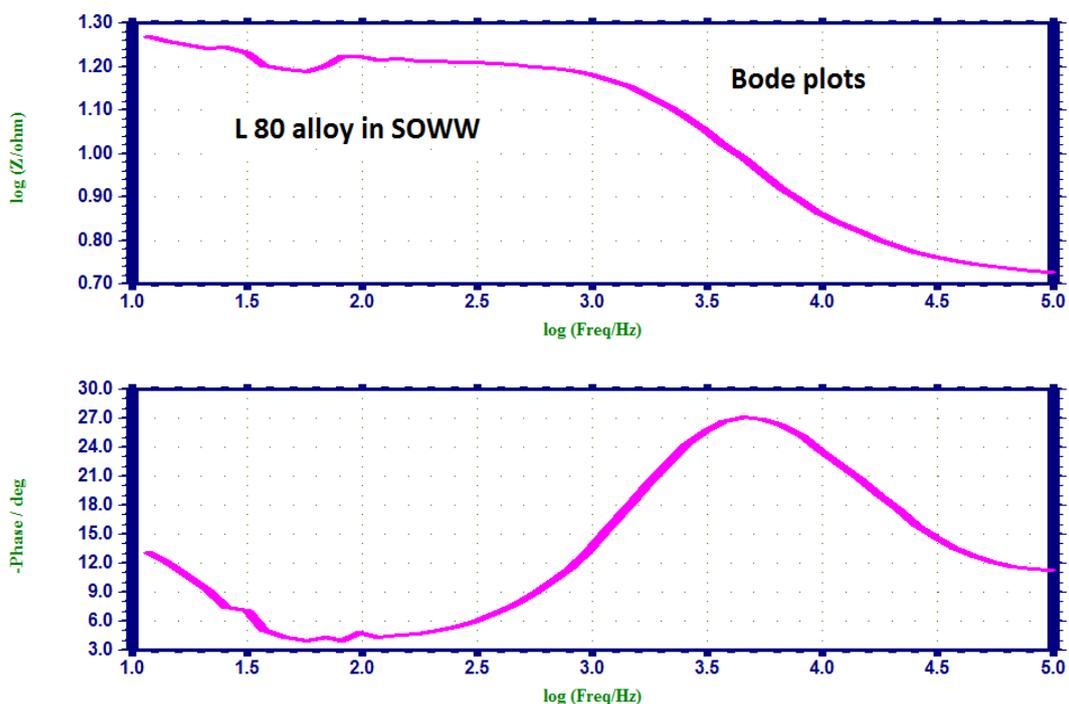
Figure 6. Bode plots of L 80 alloy immersed in SOWW
