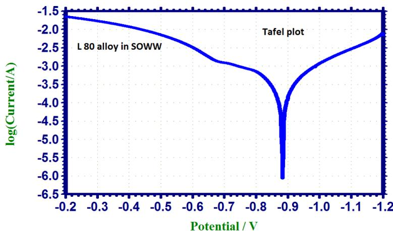
Figure 1. Polarisation curve of L 80 alloy immersed in SOWW
