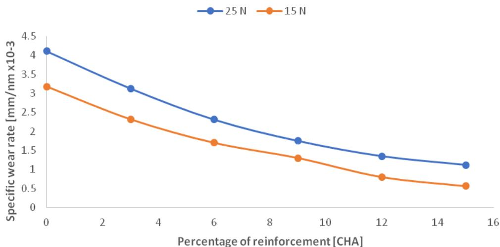
Figure 6. Effect of reinforcement on specific wear rate
