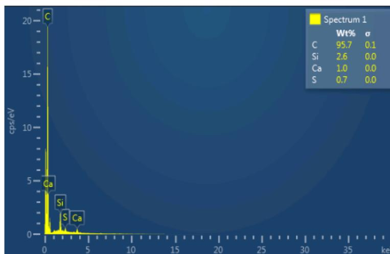
Figure 3. SEM/EDS of Cow horn ash (CHA)
