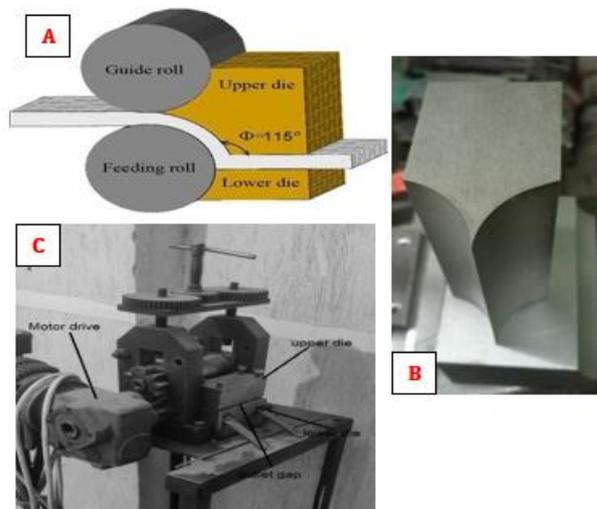
Figure 1. a) Schematic illustration of the ecar device, b) Die with angle 115°, c) The machine device used with die
