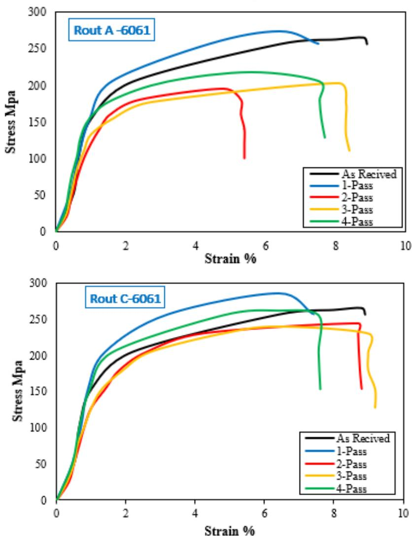
Figure 4. Al-6061 at each pass for rout A and C
