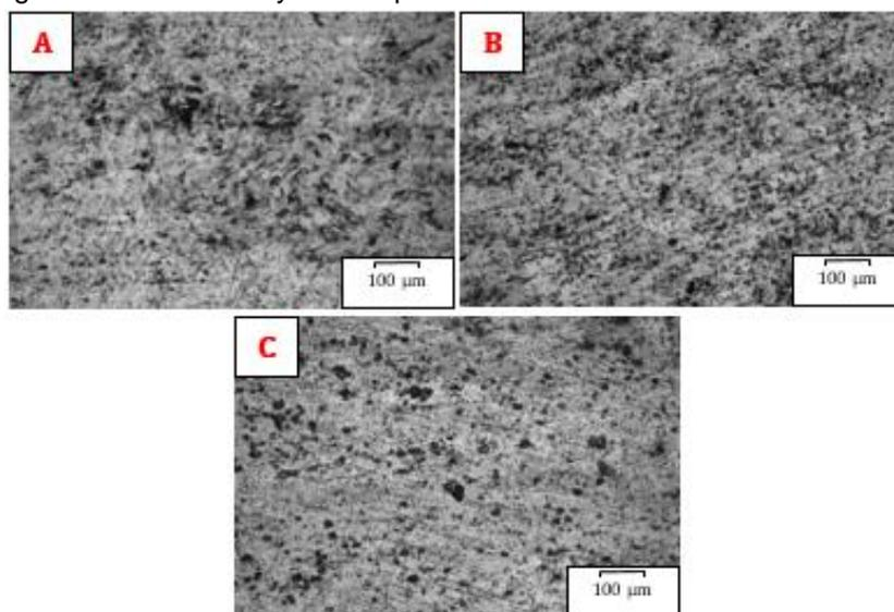
Figure 3. Optical micrograph for Al 1050 rout C a) first pass. B) six passes without annealing. C) fifth passes with annealing
