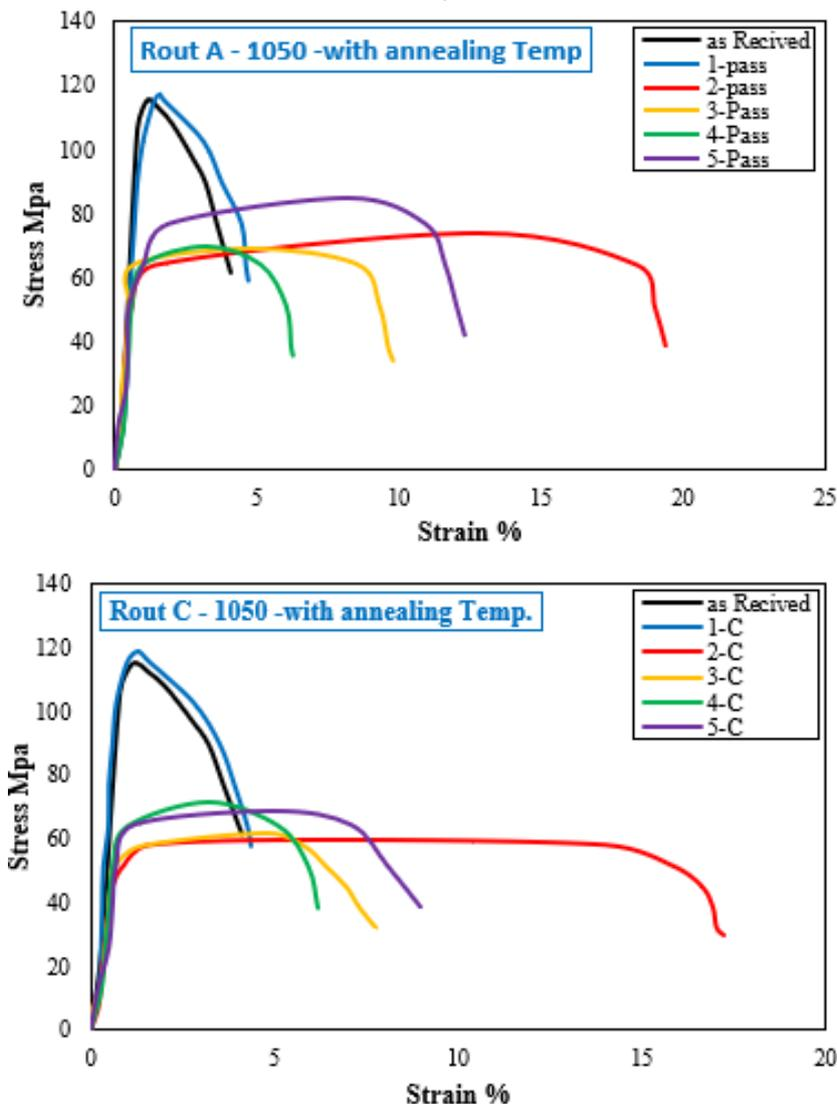
Figure 5. AL-1050 at each pass for rout A and C
