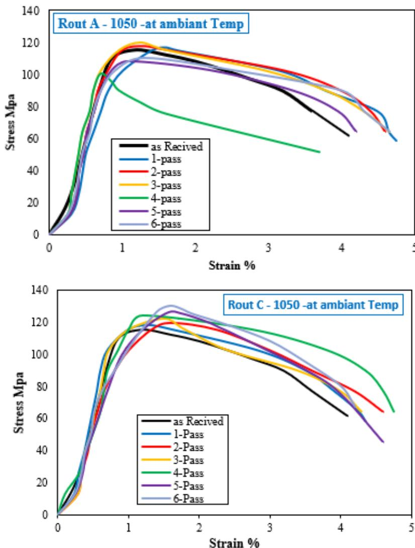
Figure 6. Al-1050 at each pass for rout A and C at ambient temperature
