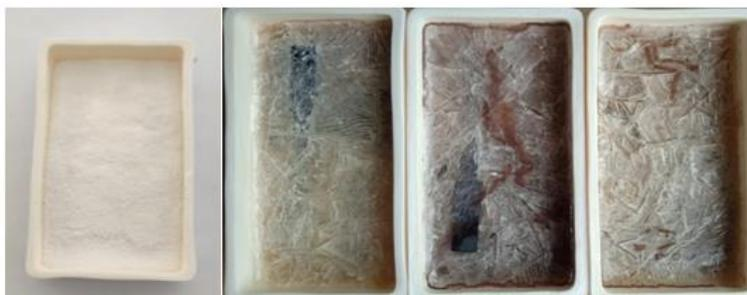
Figure -3 – Specimens in crucibles before and after the heating process
