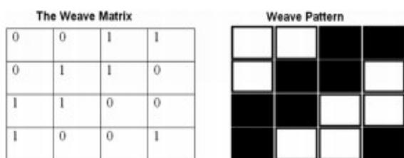
Figure 4. The weave matrix was generated from the four successive OCT scans corresponding to 2/2 twill weave pattern
