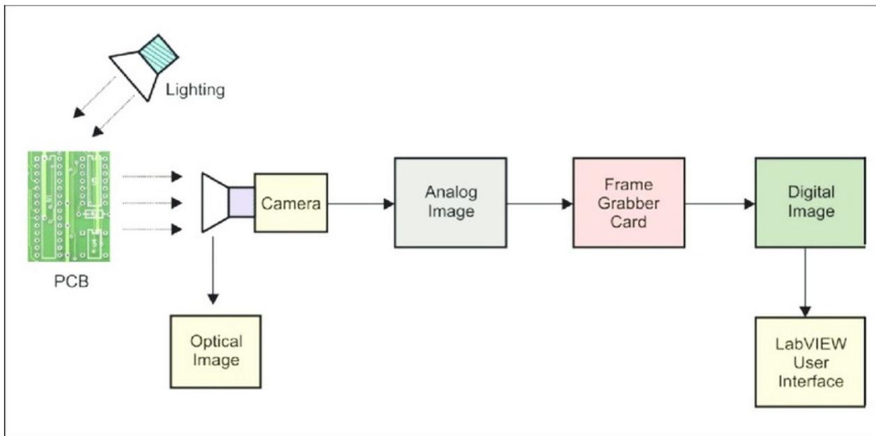
Figure 1. Schematic diagram of image processing system
