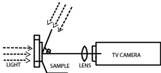
Figure 2. Geometrical arrangement to obtain the images of the woven fabric
