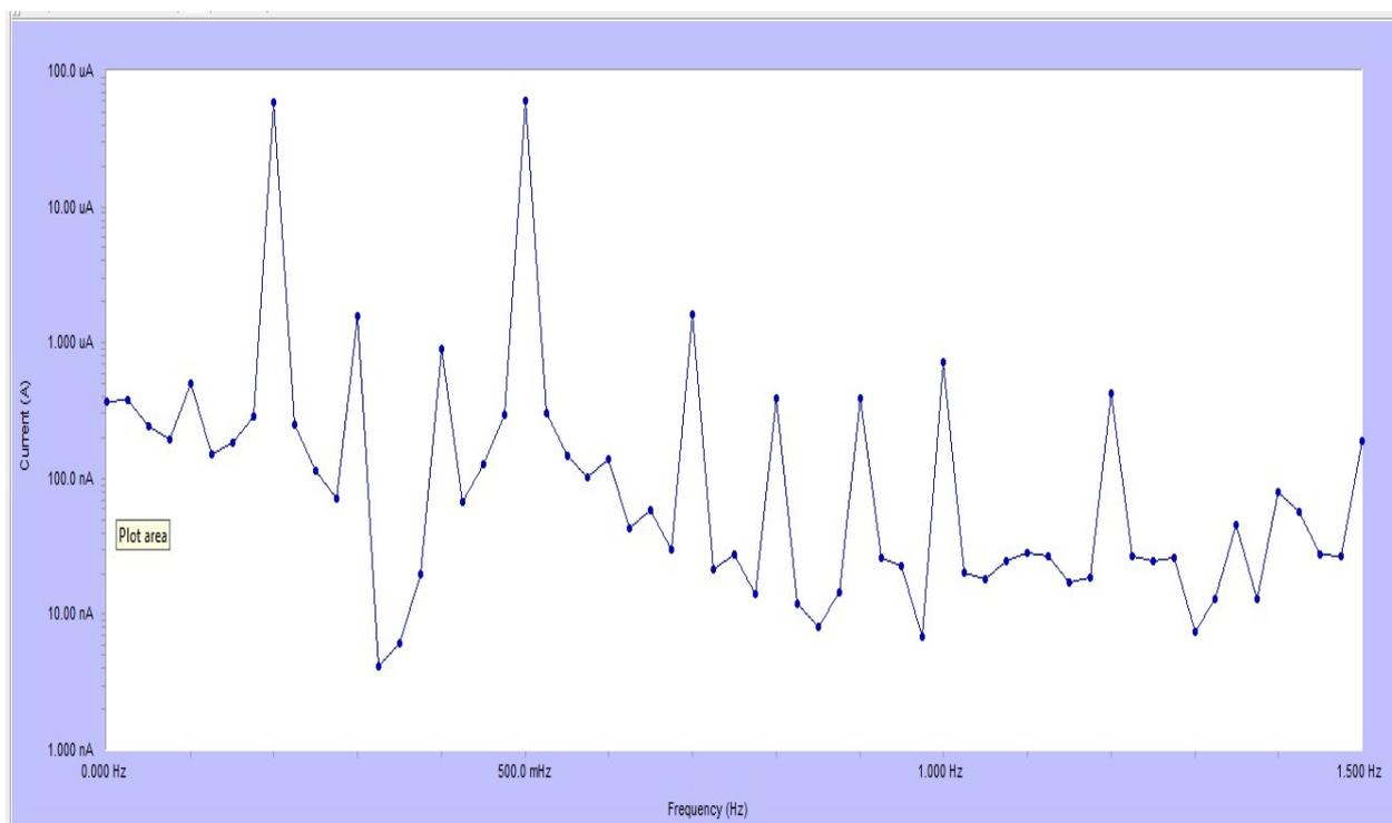
Figure 5. EFM spectra for C-steel in 1M HCl with and without  $21 \times 10^{-6} M$  of 5-Arylidene barbituric acid derivative at 25°C
