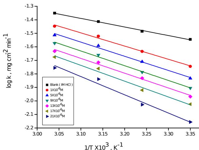
Figure 6. Log k – 1/T curves for C-steel dissolution in 1M HCl in the absence and existence of altered doses of 5-Arylidene barbituric acid derivative
