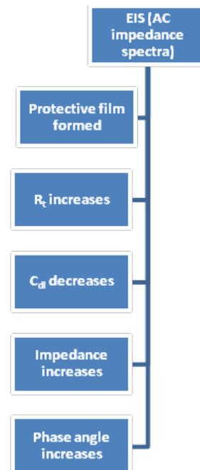
Figure 5. Correlation among corrosion parameters of AC impedance spectra
