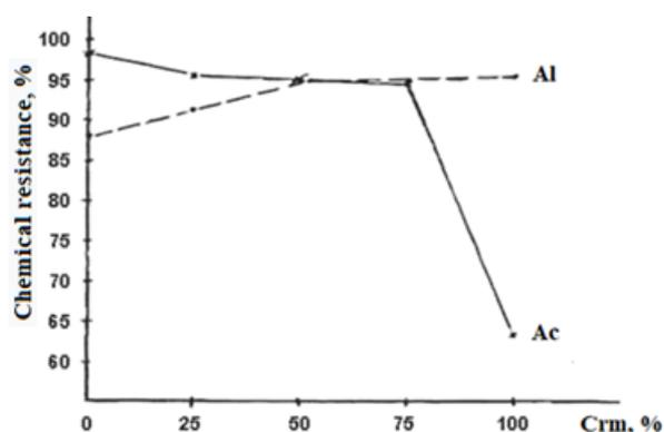
Figure 1. Dependence of acid resistance (Ac) and alkali resistance (Al) of ceramics from the concentration of red mud (Crm)
