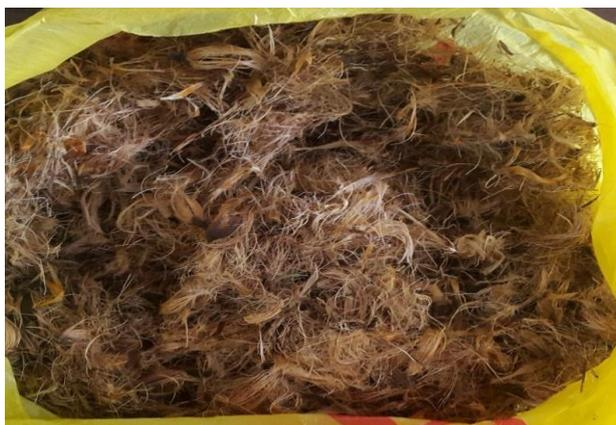
Figure 1. Dried Oil Palm Fruit Fibre.
