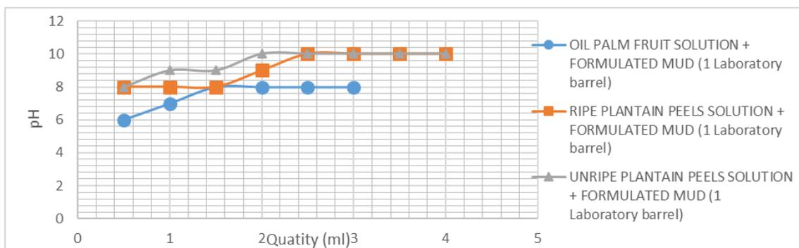
Figure 3. pH Vs Quantity, ml (Formulated Mud)
