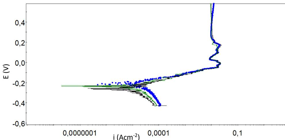
Figure 2. Potentiodynamic polarization curves of copper in 3% NaCl without and with the addition of flower extract: --- 3% NaCl; --- 3% NaCl+0,01612 gdm<sup>-3</sup>; --- 3% NaCl+0,04828 gdm<sup>-3</sup>
