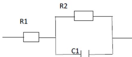
Figure 4. Scheme of the equivalent circuit of a simple electrochemical cell: C1-capacitor, R1-electrolyte resistance, R2- resistance of charge transmission
