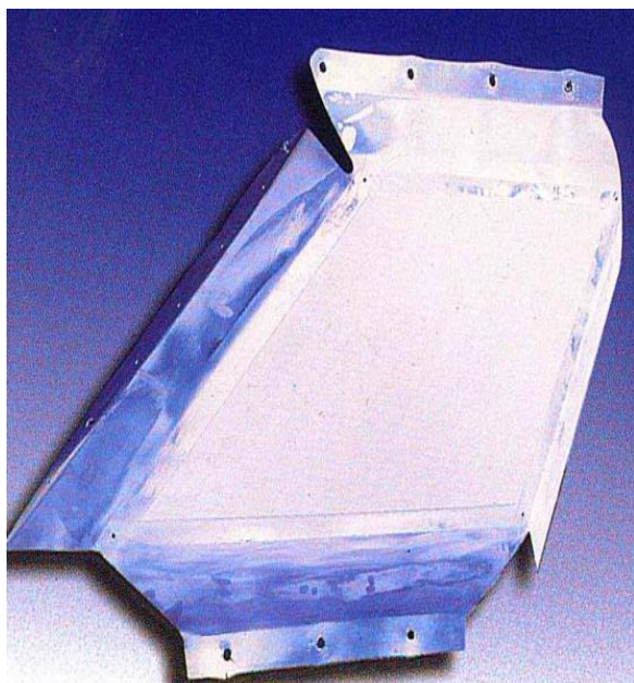
Figure 9. Section of the wing of a plane with a coating NiCr/Al/Co/Y 2 O 3 /ZrO 2 24%MgO
