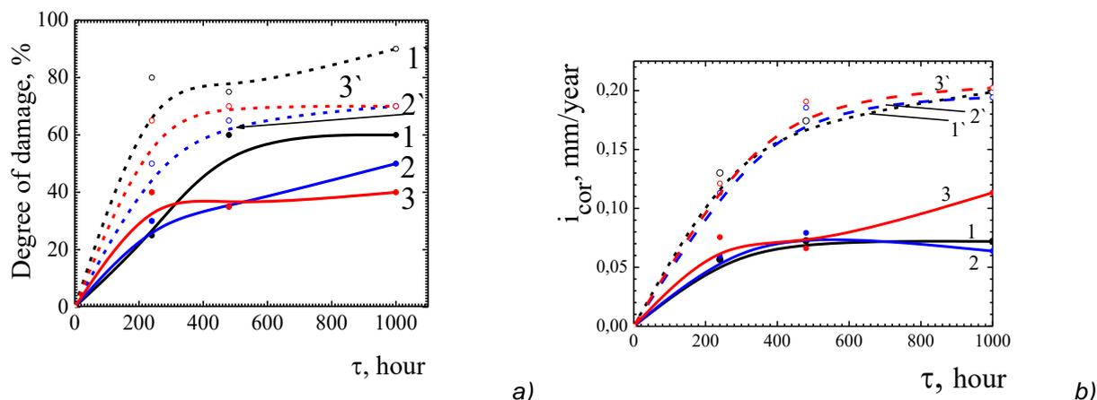
Figure 6. Degree of surface damage by corrosion (a) and corrosion resistance (b) of the base metal and welded joints of 17G1S-U steel after corrosion-mechanical tests in the 3% NaCl solution: 1, 1' is the base metal in the unstressed and stressed states; 2, 2' is the welded joint without LHT in the unstressed and stressed states; 3, 3' is the welded joint after LHT in the unstressed and stressed states
