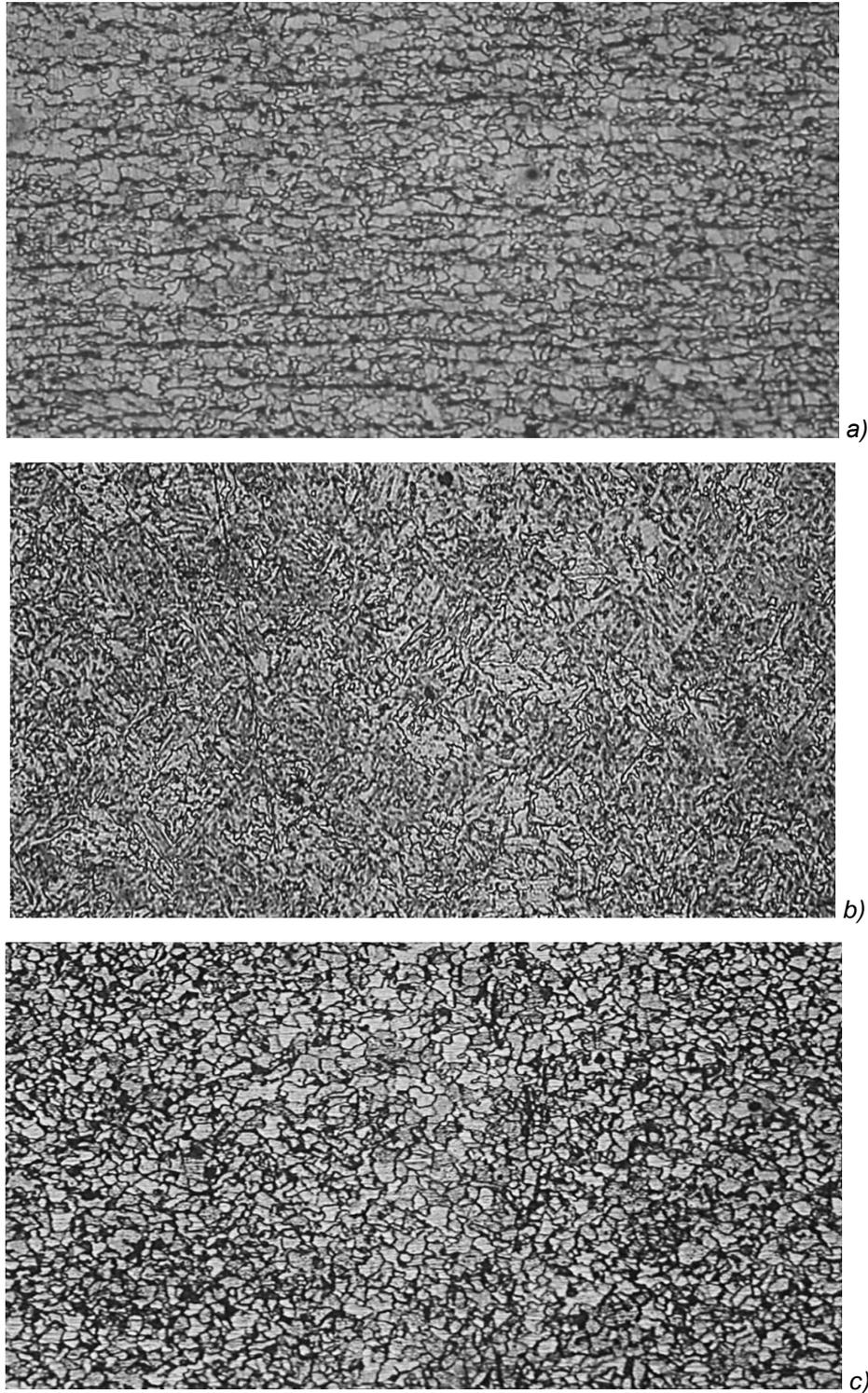
Figure 1. Microstructure of different zones of HF welded joints of 17G1S-U steel:
