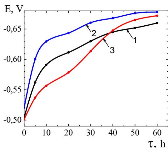
Figure 2. Change of corrosion potential with time, measured in different zones of welded joints: 1 – base metal, 2 – welded joint without LHT, 3 – welded joint after LHT.
