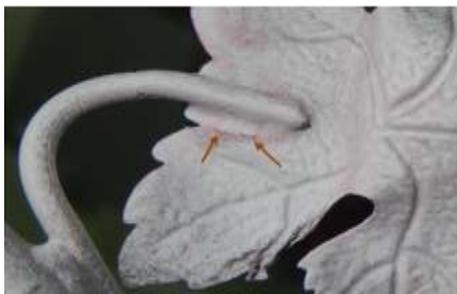
Figure 5. Enlarged view of discovered crack (≈6mm in length) at leaf
