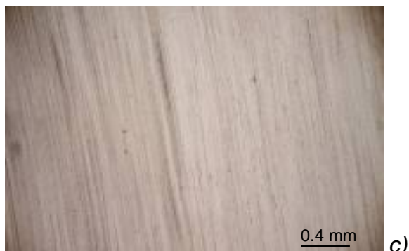
Figure 3. Light microscopy images of the electrode surfaces after cyclic polarization measurements for a) AISI 304, b) AISI 316L and c) duplex stainless steel
