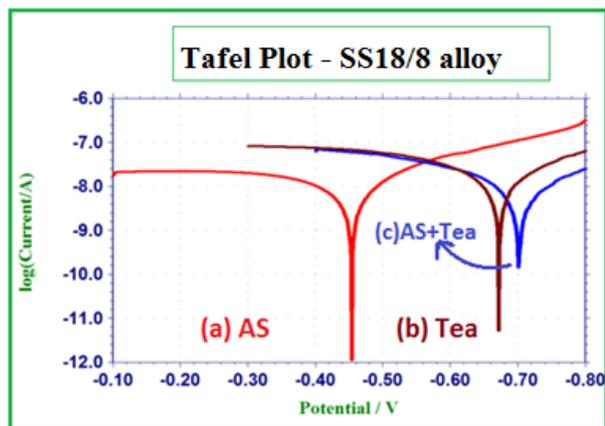
Figure 2. Polarization curve of SS18/8 alloy immersed in various test solution: (a) AS (b) Tea (c) AS + Tea
