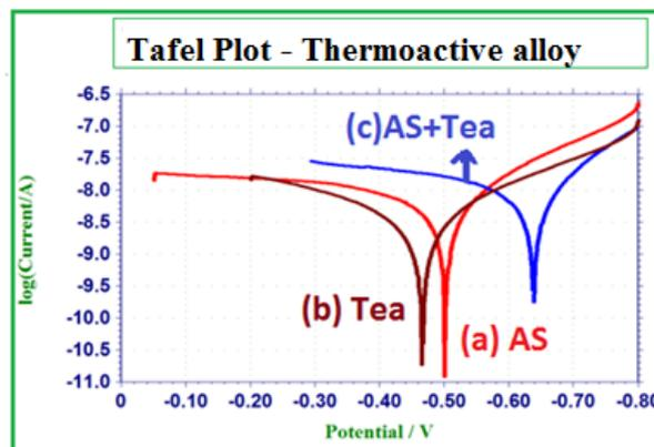
Figure 3. Polarization curve of Thermoactive alloy immersed in various test solution: (a) AS (b) Tea (c) AS + Tea
