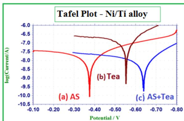
Figure 1. Polarization curve of Ni-Ti alloy immersed in various test solution: (a) AS (b) Tea (c) AS + Tea
