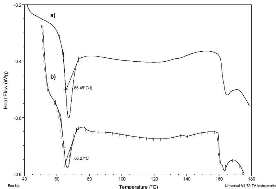
Figure 13. DSC thermograms of poly(Aam-co-Aac) hydrogel 70:30 (Aac:Aam) with 1% of crosslinking agent synthesized using the: a) APS, b) KPS as initiator
