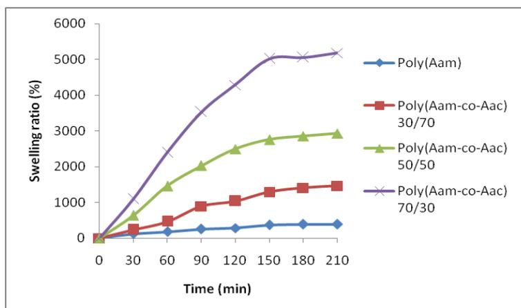
Figure 4. Swelling behaviour of KPS initiated poly(acrylamide-co-acrylic acid) hydrogels with 3% crosslinking agent in alkaline medium (pH=10)
