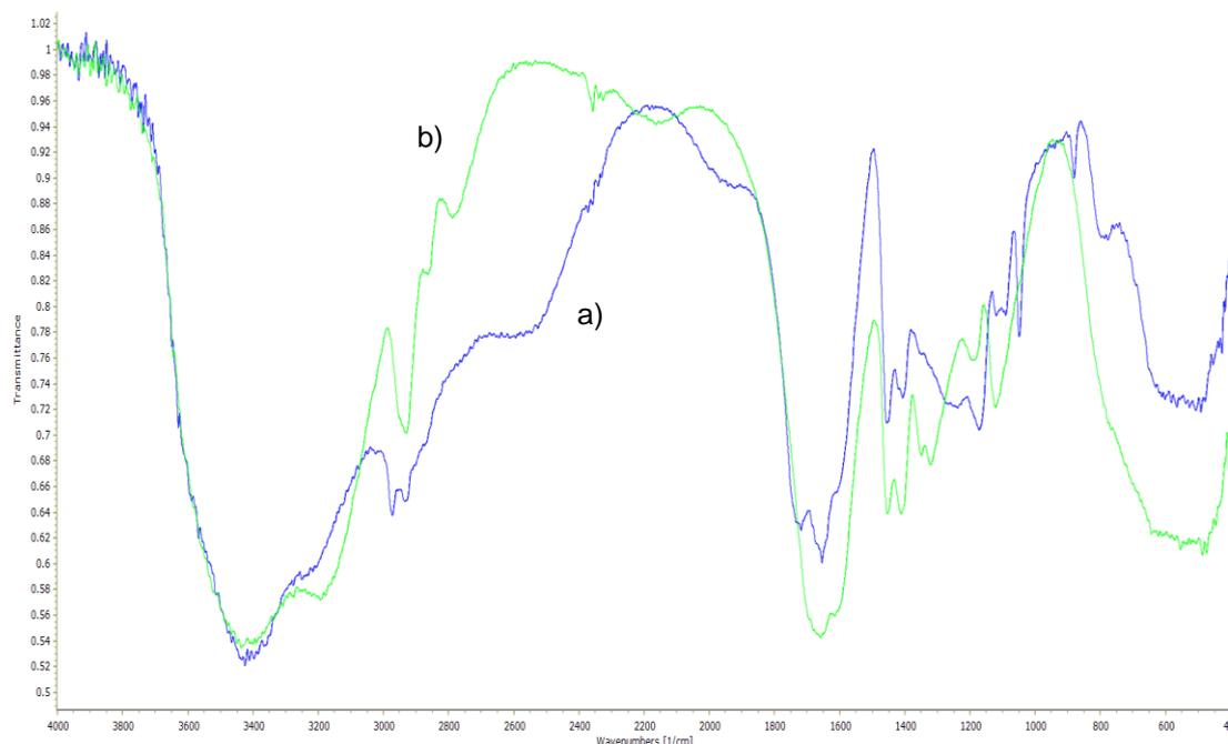
Figure 2. FT-IR spectra of poly(Aam-co-Aac) 50:50 hydrogel (a line) and poly(Aam) hydrogel (b line)
