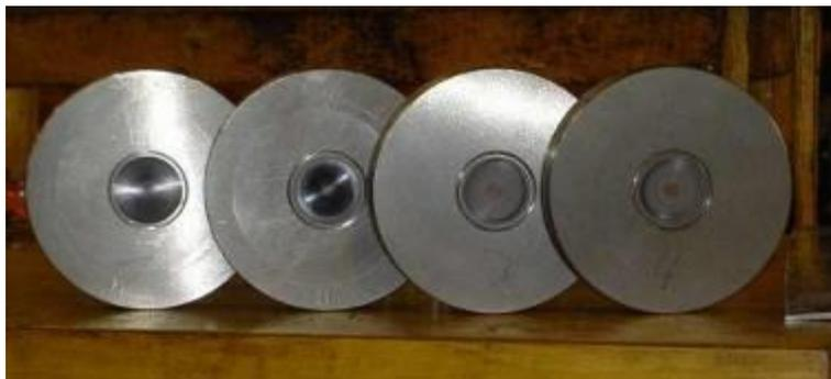
Figure 2.  $\text{Si}_3\text{N}_4$  test samples
