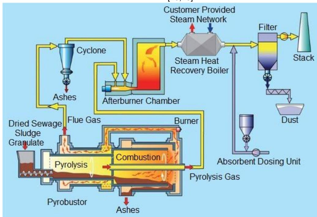
Figure 1. The process of pyrolysis of sewage sludge [27].
