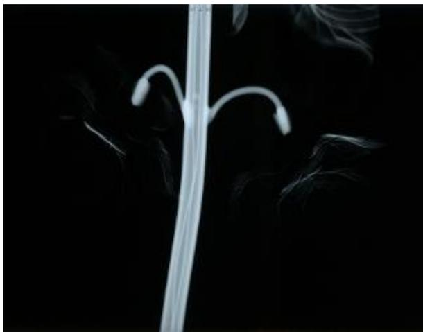
Figure 5. X-ray film of central part of desk lamp with leaves ( $\approx 1\text{mm}$  in thickness)
