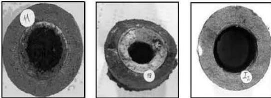
Figure 4. Macro appearance of SEN with build-up formed on the internal SEN wall, but without the appearance of internal erosion.
