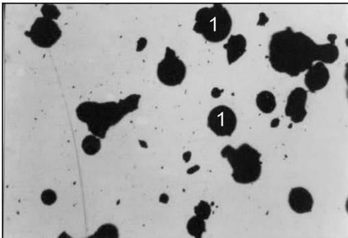
Figure 9. Micrograph of granulated casting powder (transmitted light), magnification x250; 1-granules
