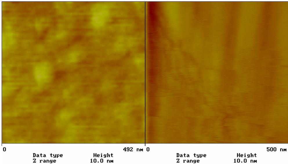
Fig.5 AFM image of (a) fresh glass surface, (b) glass surface coated with thin polymer layer . Roughness analysis:  $R_q=0,48$  nm,  $R_a=0,36$  nm for (a) and  $R_q=0,24$  nm,  $R_a=0,17$  nm for (b).
