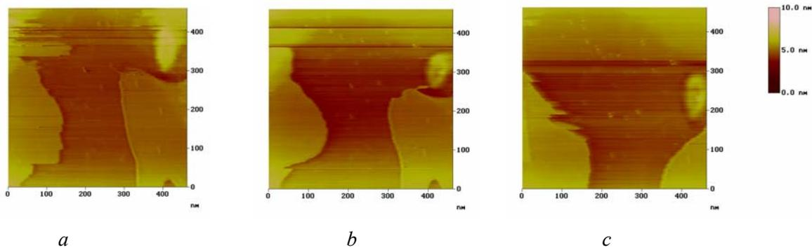
Fig. 3 - In-situ STM observation of the dissolution of the Ni layer in 0.01 M  $H_2SO_4$ . Series of constant-current in-situ STM images of Ni electrode recorded at constant potential 1,1 V and tunneling current 5nA. (a) – fresh electrodeposited Ni electrode, (b) and (c) – after 5 and 10 min, respectively.
