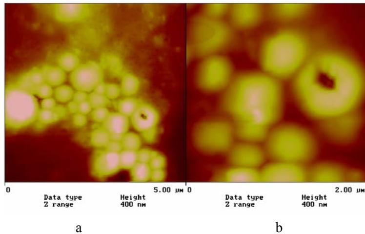
Fig.2 Corrosion of zirconium layer deposited on iron. AFM images of the same region; scan range (a) 5000 nm and (b) 2000 nm. Roughness analysis:  $R_q=72,7$  nm,  $R_a=58,8$  nm for (a) and  $R_q=47,8$  nm,  $R_a=38,2$  nm for (b).
