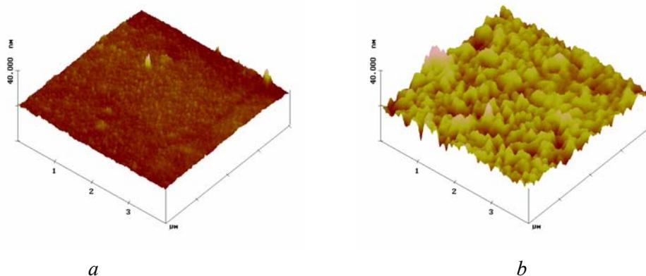
Fig. 4 - The long-term atmospheric corrosion of stained glass.
