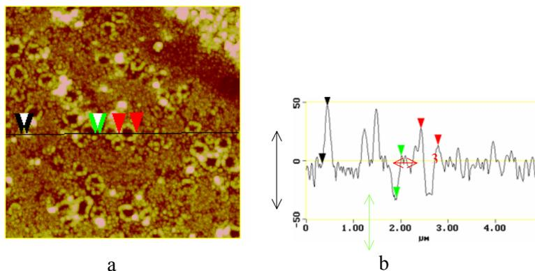
Fig.1 - AFM image (5000x5000x200 nm) of corroded Ni layer deposited on iron (a). Section analysis (b) shows the height profile along the line chosen on Fig.1a. Roughness analysis:  $R_q$  (RMS) =13.3 nm,  $R_a$  (mean roughness) =9,1 nm.
