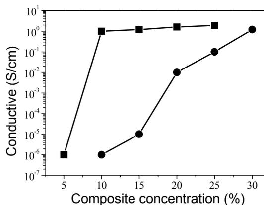
Figure 1 - Electric conductivity curves vs composition concentration for KPO (■) and KP20 (●)
