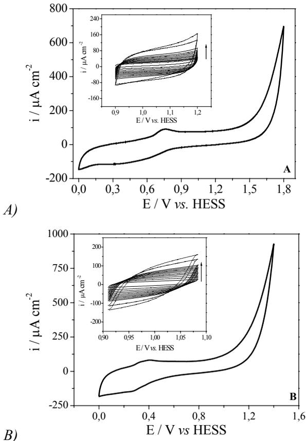
Figure 2 - Cyclic voltammetry studies for (A) KPO and (B) KP20 composites in  $0.5 \text{ mol L}^{-1} \text{ H}_2\text{SO}_4$  solution.  $\nu = 10 \text{ mVs}^{-1}$ . The inserts shows the double-layer responses for both materials
