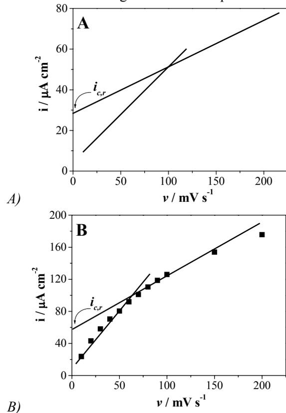
Figure 3 - Linear dependence of the capacitive currents in function of the scan rates for (A) KPO and (B) KP20 composites. The capacitive current values were obtained directly by the Fig. 2.
