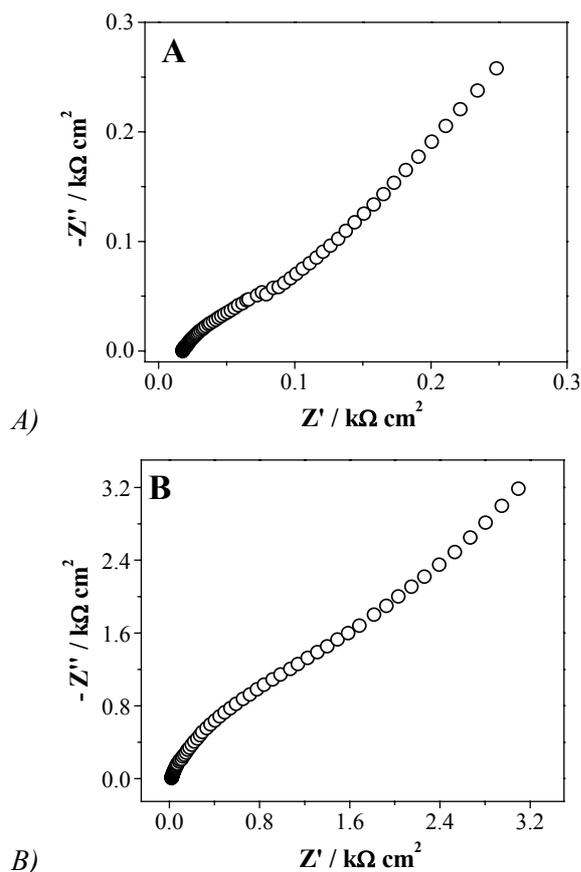
Figure 4 - Nyquist plots for (A) KPO and (B) KP20 in  $10^{-3} \text{ mol L}^{-1} \text{ K}_4\text{Fe}(\text{CN})_6 + 0,5 \text{ mol L}^{-1} \text{ H}_2\text{SO}_4$  solution. The measurements were carried out with fixed potentials of 0,7 V and 0,3 V for KP20 and KPO.
