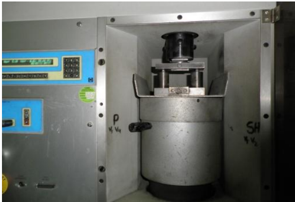
Figure 8 - Mercury intrusion porosimeter used for porosity measurement
