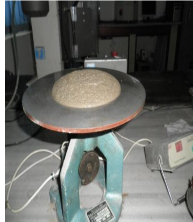
Figure 4 - The flow table used for the flow measurements
