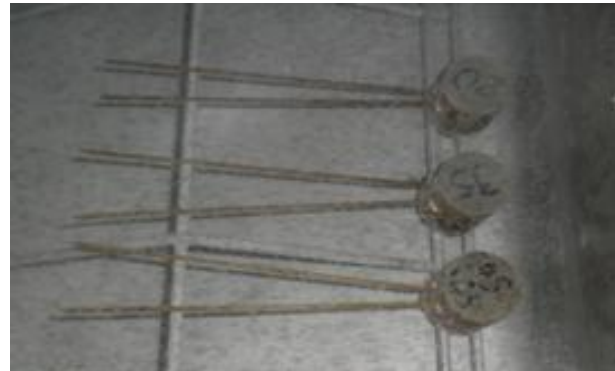
Figure 5 - Le Chatelier rings used for the autoclave tests
