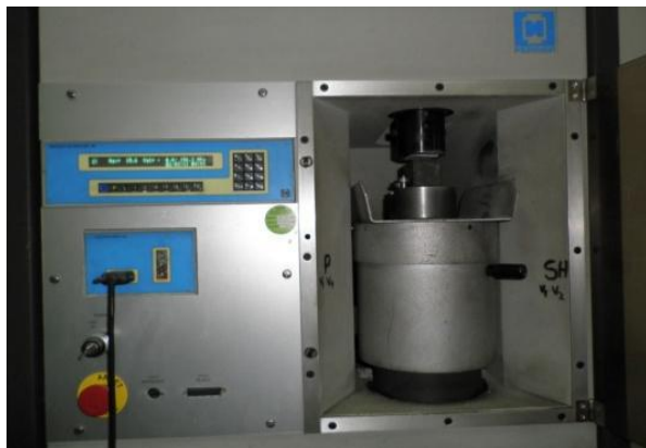
Figure 6 - The apparatus used for flexure and compressive strength measurements
