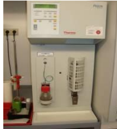
Figure 8 - Mercury intrusion porosimeter used for porosity measurement
