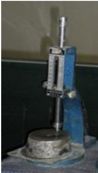
Figure 3 - Vicat apparatus used for normal consistency and setting time determination
