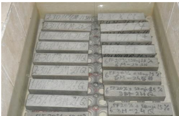
Figure 7 - The prisms cured for sulfate resistance measurements
