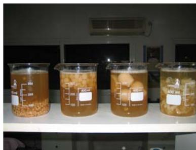
Figure 8 - Treatment of waste waters using 100 g of yeast beads with different dimensions. The dimensions of these beads as shown in the figure are: 1-2 mm; 1-2 cm; 5-7 cm; filamentous
