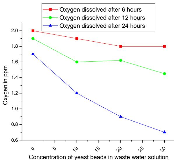
Figure 6 - Oxygen content in waste waters after treatment of 1000 ml water effluents with continuous mixing 100 rpm in aerobic conditions. Time of measurements after 6, 12 and 24 hours with concentration of yeast beads respectively 0%; 10%; 20% dhe 30%.
