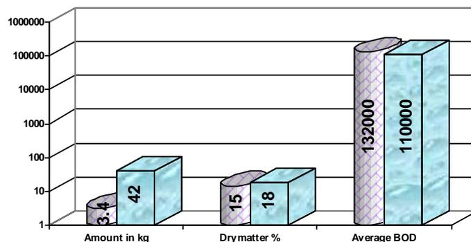
Figure 2. Slurry characteristics in brewing process
