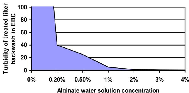
Figure 6 - Water turbidity after filter backwash treatment
