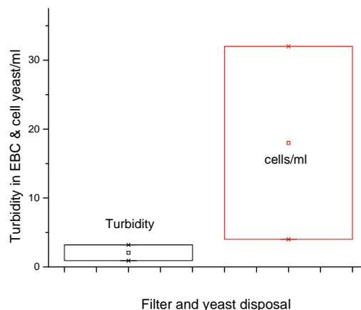
Figure 4. Turbidity of spent yeast effluent after alginate treatment (4%) and cell yeast number in slurry
