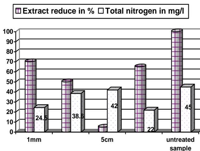
Figure 9 - Extract reduction and total nitrogen for different beads used in weak wort treatment procedure
