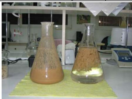
Figure 3 - In the left slurry from filter effluent, in the right gel entrapment of the slurry in alginate
