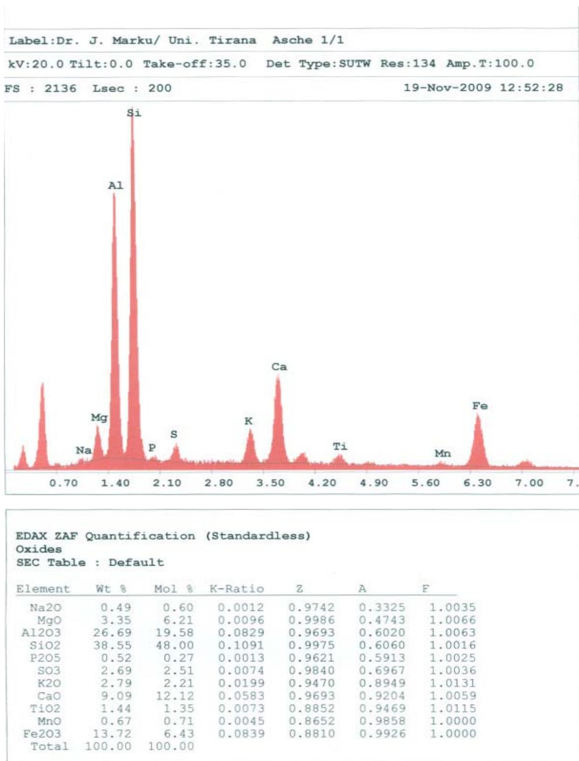
Figure 2 - EDAX spectrum for representative sample of fly ash FA<sub>1</sub>
