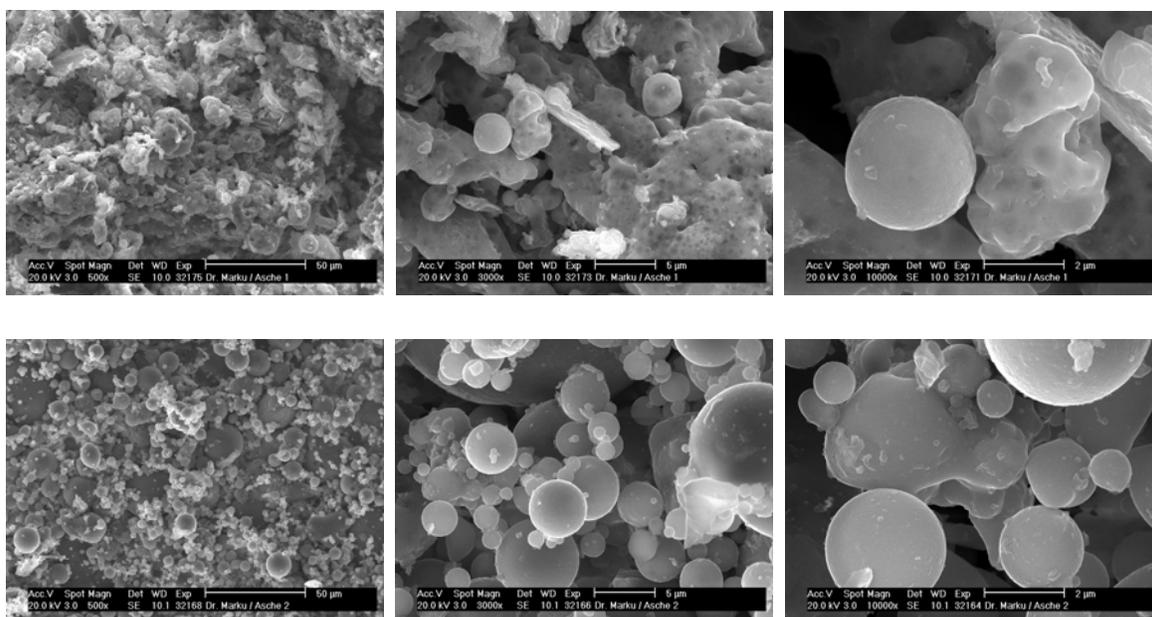
Figure 1 - SEM micrographs of two different fly ashes (above for fly ash FA1 and below for fly ash FA2)
