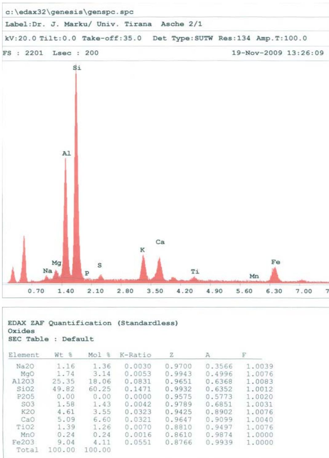
Figure 3 - EDAX spectrum for representative sample of fly ash FA<sub>2</sub>
