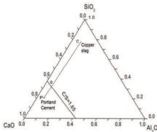
Figure 1 - The phase diagram for the ternary system  $CaO-Al_2O_3-SiO_2$ , with plotted Portland cement and copper slag, the line (PC) representing their mixing ratios and point (O) where, based on zero CH, the optimum mixture ratio lies
