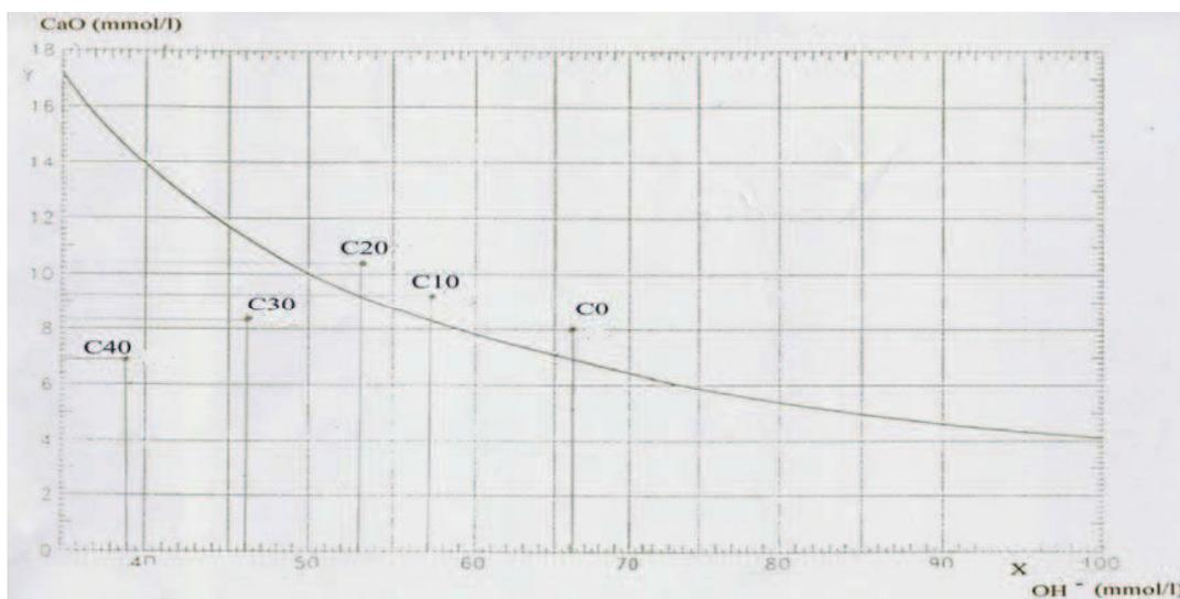
Figure 2 - Solubility of  $\text{Ca}(\text{OH})_2$  in solution of alkali hydroxides at 40°C
