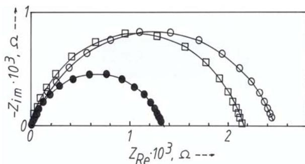
Figure 7 - Experimental ( $\circ$ ;  $\bullet$ ;  $\square$ ) and theoretical (—) Nyquist plots for austenitic steel 316L (weld -  $\circ$ -; OHZ -  $\bullet$ - and BM -  $\square$ -) in deaerated 15 % (1.7 M) H<sub>2</sub>SO<sub>4</sub> at 0.3 V/she and room temperature using R(QR)-EEC.
