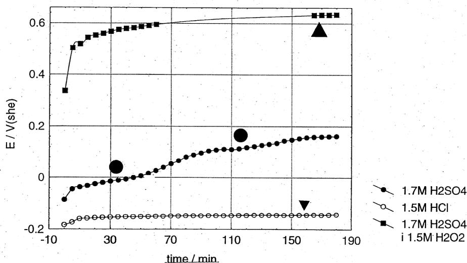
Figure 4 - OCP / time - dependences for spontaneous passivation of steel 316 L in several deaerated acidic solutions, basic material - zone 3 (after cathodic pretreatment at - 0.25 V/she for 10 min.), room temperature.
