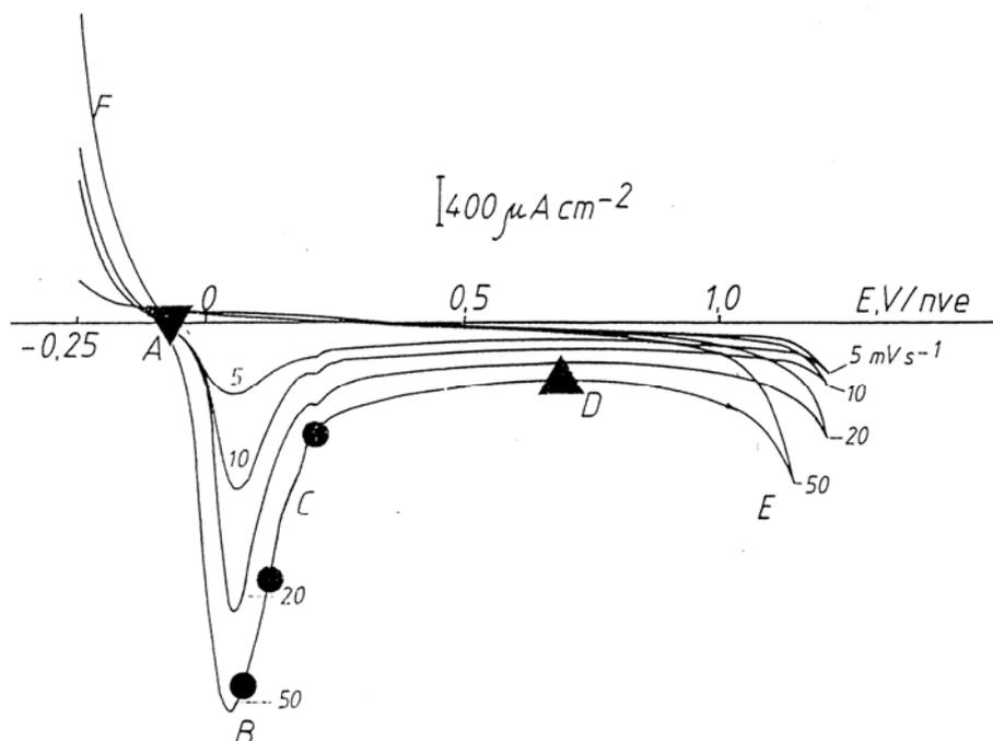
Figure 3 - Cyclic voltammograms for electrochemical passivation of austenitic steel 316 L, basic material – zone 3 in 1.7 M  $H_2SO_4$ , at room temperature.
