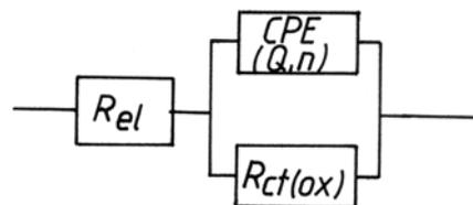
Figure 5 - Equivalent electric circuit for impedance characterization of metal/solution and metal/oxide/solution-interface.
