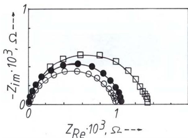
Figure 6 - Experimental ( $\circ$ ;  $\bullet$ ;  $\square$ ) and theoretical (—) Nyquist plots for austenitic steel 316L (weld -  $\circ$ -; OHZ -  $\bullet$ - and BM -  $\square$ -) in deaerated 15 % (1.7 M) H<sub>2</sub>SO<sub>4</sub> at -0.15 V/she and room temperature using R(QR)-EEC.
