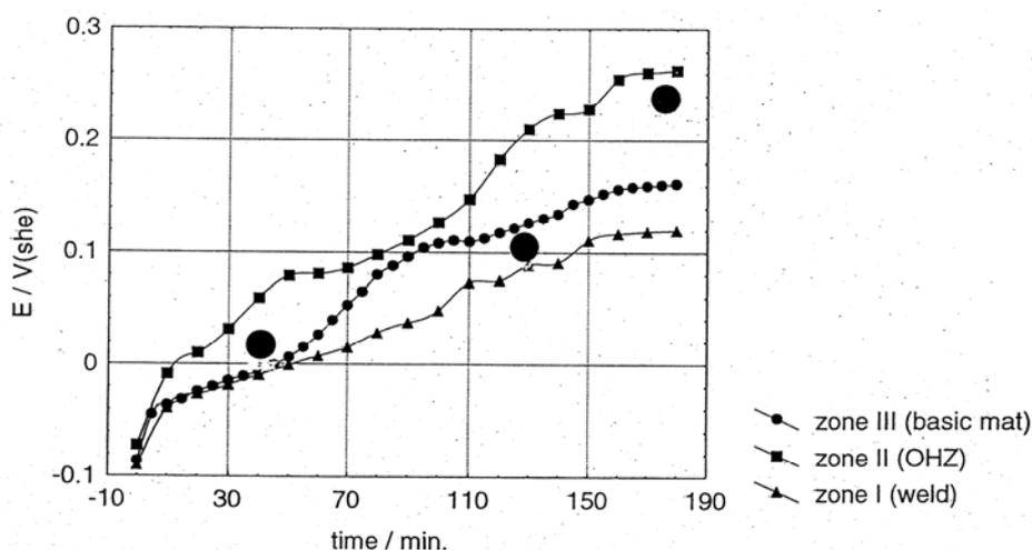
Figure 2 - OCP / time - dependences for spontaneous passivation of steel 316 L in deaerated  $1.7$  M  $\text{H}_2\text{SO}_4$  (after cathodic pretreatment at  $-0.25$  V/she for 10 min.) at room temperature.
