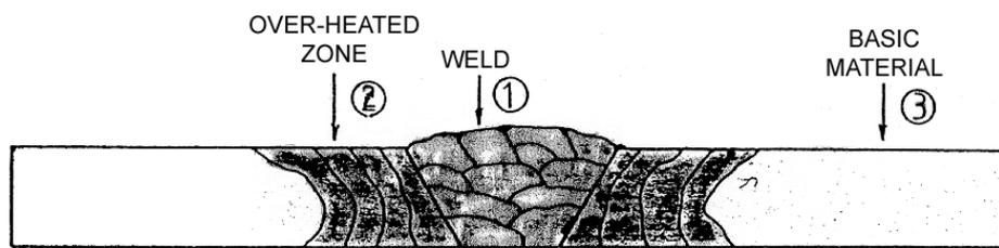
Figure 1 - Schematic representation of welded part (steel 316 L): weld - zone 1; overheated zone – zone 2 and basic material – zone 3.
