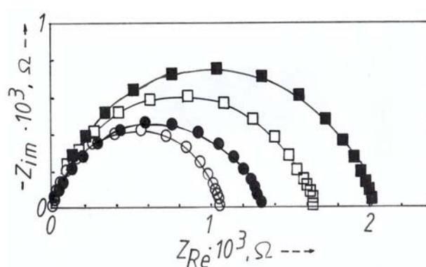
Figure 8 - Experimental ( $\circ$ ;  $\bullet$ ;  $\square$ ;  $\blacksquare$ ) and theoretical (—) Nyquist plots for austenitic steel 316L (OHZ) in deaerated 15 % (1.7 M) H<sub>2</sub>SO<sub>4</sub> at -0.15 (-  $\circ$ -); 0.3 (-  $\bullet$ -); 0.7 (-  $\square$ -) and 0.9 (-  $\blacksquare$ -) V/she and room temperature using R(QR)-EEC.
