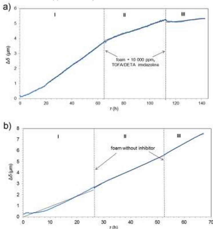
Figure 7 - Time dependence of metal thickness loss for mild steel set in vapor phase after being contacted by the foam plug a) without and b) with 10 000 ppm<sub>v</sub> of TOFA/DETA imidazoline.
