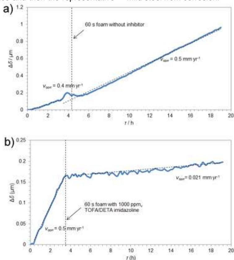
Figure 6 - The time dependences of metal thickness loss for mild steel in vapor phase, contact time 60 s with foaming agent a) without and b) with 1000 ppm<sub>v</sub> TOFA/DETA imidazoline (3 wt. % NaCl solution, at 70°C, pH 4 with acetic acid in a concentration of 0.02 mol dm<sup>-3</sup>).
