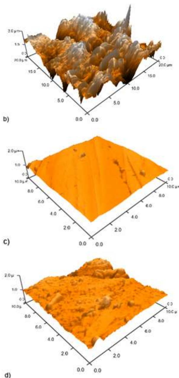
Figure 5 - Atomic force microscopy three-dimensional images of mild steel surface in 3 wt. % NaCl saturated with CO<sub>2</sub> a) without inhibitor at 20°C, b) without inhibitor at 70°C, c) containing 70 ppm<sub>v</sub> TOFA/DETA imidazoline at 20°C and d) containing 70 ppm<sub>v</sub> TOFA/DETA imidazoline at 70°C. (Reprinted with permission from [19] Copyright 2013 Elsevier).
