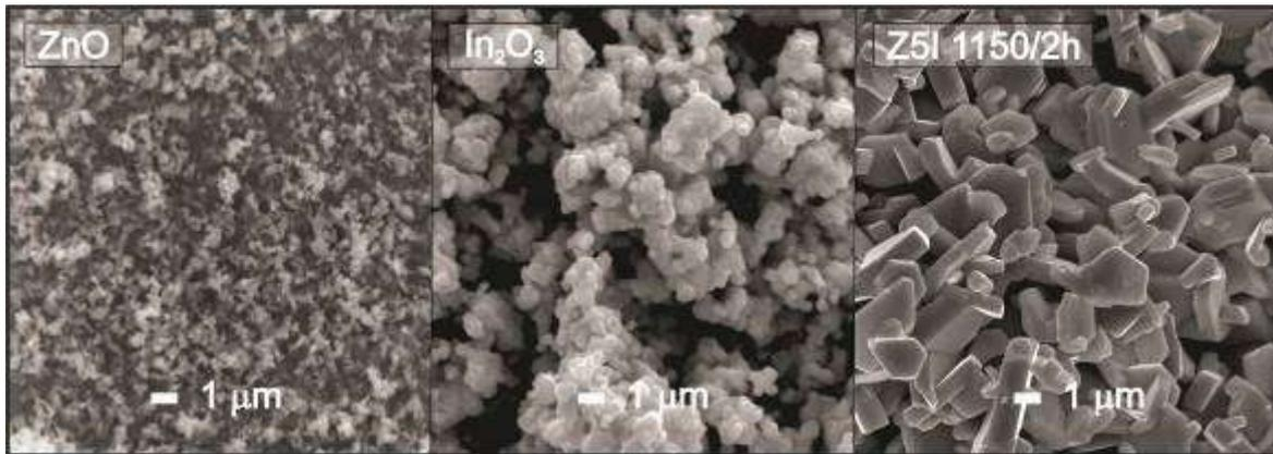
Figure 2 - SEM images of the starting ZnO and  $\text{In}_2\text{O}_3$  powders, and the powder with composition  $(\text{ZnO})_5\text{In}_2\text{O}_3$  pre-reacted in loose form at  $1150^\circ\text{C}$
