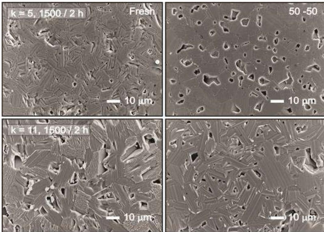
Figure 3 - Thermally etched microstructures of the  $(\text{ZnO})_k\text{In}_2\text{O}_3$  ( $k=5,11$ ) ceramics, prepared from the fresh powder mixtures of ZnO and  $\text{In}_2\text{O}_3$  (fresh) or starting mixture containing also pre-reacted powder (50-50), sintered at  $1500^\circ\text{C}$  for 2 hours.
