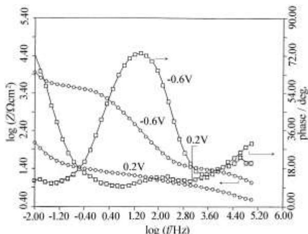
Figure 2 - Bode – plots ( $\log Z - \log f$ , and  $\phi - \log f$ ) for PPy film ( $5 \mu\text{m}$ ) in doped ( $E = 0.2 \text{ V/SHE}$ ) and undoped ( $E = -0.6 \text{ V/SHE}$ ) states, in  $0.5 \text{ mol dm}^{-3} \text{ NaClO}_4 / \text{ACN}$  solution [101].
