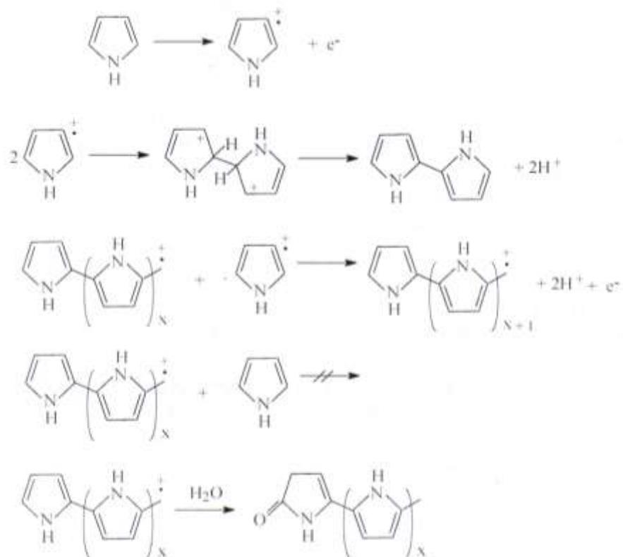
Scheme 1 - Electrochemical polymerization of pyrrole [48].
