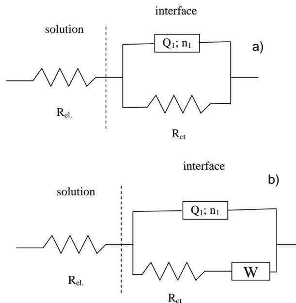
Figure 4 - Electrical equivalent circuits for undoped ( $E = -0.6$  V/SHE) state of PPy in the PPy / AC - composite film with 30 wt% of AC in the polymerization solution; (a)  $L_{PPy} < 2.5 \mu m$ , (b)  $L_{PPy} \geq 2.5 \mu m$  [100].
