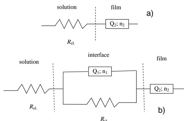
Figure 3 - Electrical equivalent circuits for doped ( $E = 0.2 \text{ V/SHE}$ ) state of PPy in the PPy / AC – composite film with 30 wt% of AC in the polymerization solution; (a)  $L_{\text{PPy}} < 2.5 \mu\text{m}$ , (b)  $L_{\text{PPy}} \geq 2.5 \mu\text{m}$  [100].
