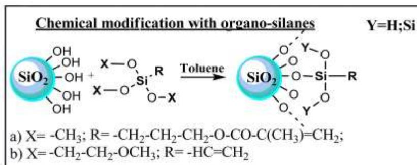
Figure 1 - Chemical modification of AEROSIL<sup>®</sup> 380 with a) TMSPM and b) TMEVS
