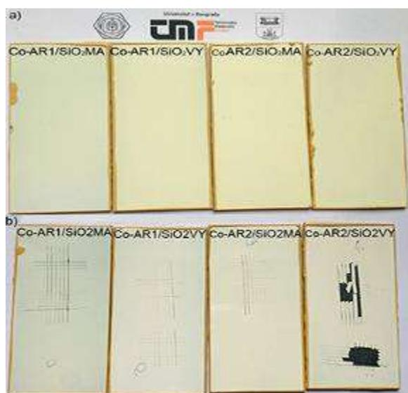
Figure 8 - Dry ARs anticorrosion coating films: Co-AR1/SiO<sub>2</sub>MA, Co-AR1/SiO<sub>2</sub>VY, Co-AR2/SiO<sub>2</sub>MA and Co-AR2/SiO<sub>2</sub>VY a) before and b) after anticorrosion analysis in humid chamber
