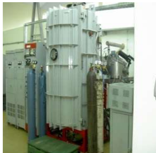
Figure 7 - PVD chamber (VU 1100) in Plasma facility
