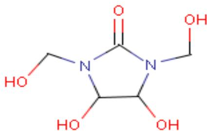
Figure 3 - Schematic presentation of DMDHEU-
