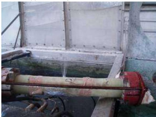
Figure 4 - Start of the pipe leakage
