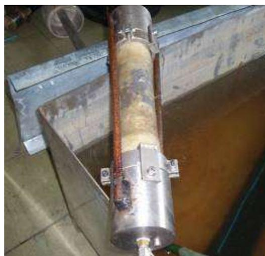
Figure 2 - "Caps" with additional welded bars as reinforcement
