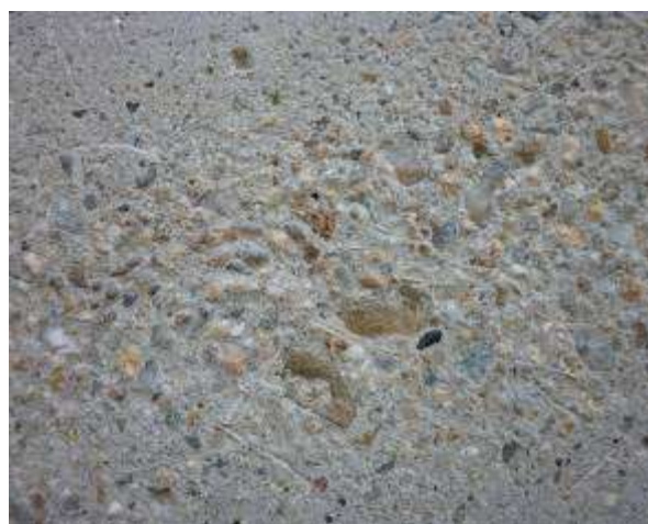
Figure 7 – The surface of the concrete sample micro-reinforced with steel fibers ZS/N – 0,50x30mm: 1 – fiber indentation, 2 – fiber cutting
