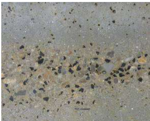
Figure 6 – Appearance of the surface of the sample of ER batch after testing of hydro-abrasion resistance
