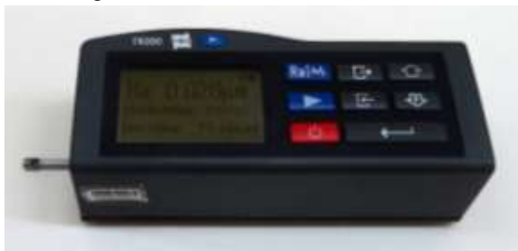
Figure 3 - Determination of surface roughness of coated surface using contact stylus surface roughness tester
