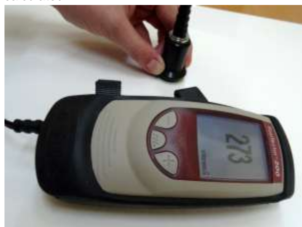
Figure 4 - Determination of dry film thickness of coating by ultrasonic gauge
