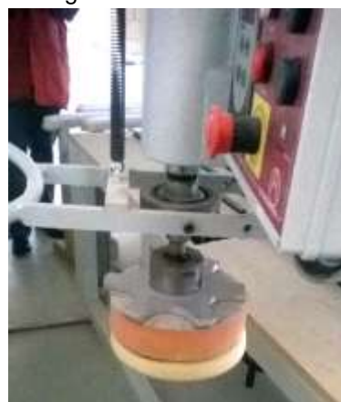
Figure 2 - Polishing disk on the hand-operated polishing machine
