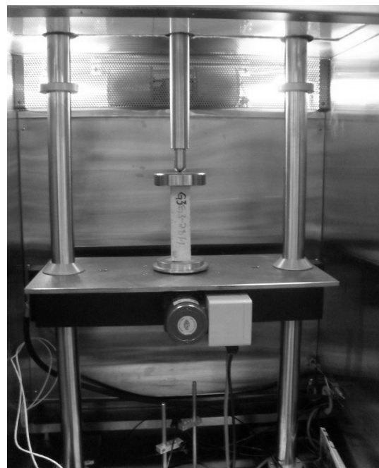
Figure 3 - Determination of modulus of elasticity ( E )
