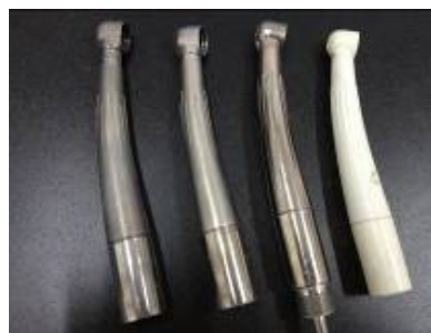
Figure 3 - Polyetherimide dental tools. Ti-coated (the first three samples from the left side) vs. uncoated tool (one sample on the right side)
