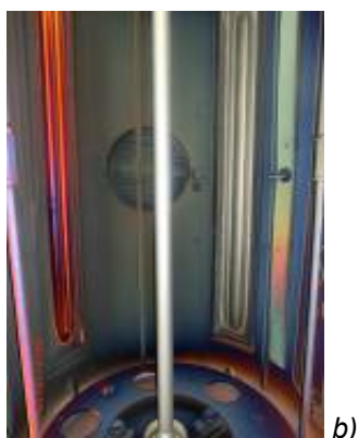
Figure 1 - PVD chamber: a) chamber with control boards for operation of the chamber, b) inner view of the targets inside the chamber
