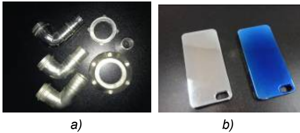
Figure 4 - PET samples coated with: a) Ti- PVD deposited coatings for different purposes, b) \text{TiO}_2 deposited coatings for decorative purpose
