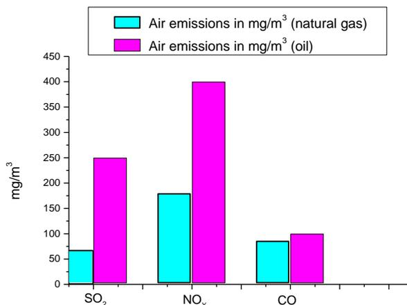
Figure 5 - Air emissions parameters at boiler outlet
