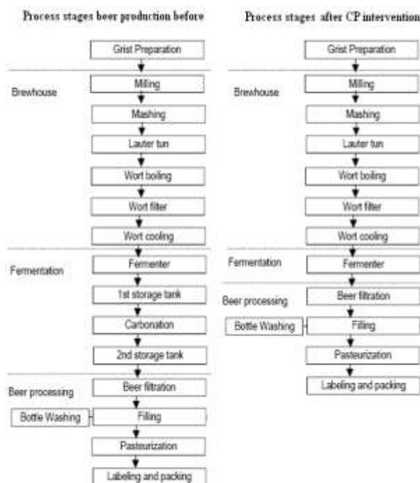
Figure 7 - Beer production diagram before and after intervention
