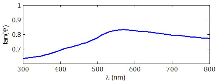
Figure 3 - Trajectories of  $tg(\psi)$  for gold 585 strip, annealed, specimen (1);
