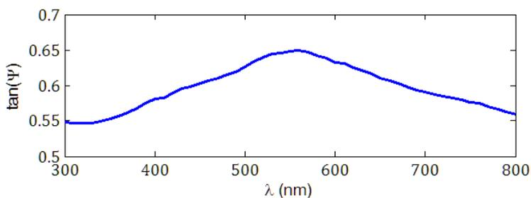
Figure 5 - Trajectories of  $tg(\psi)$  for gold 585 strip, 20% deformation, specimen (3)
