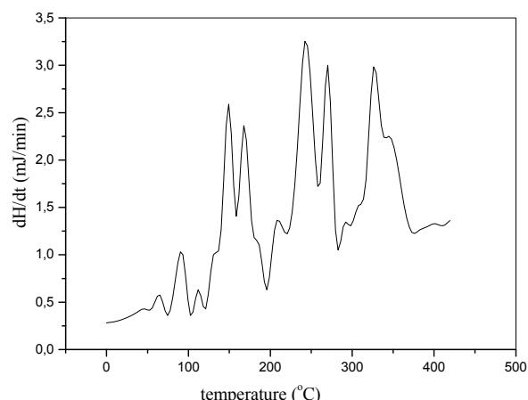
Fig. 2 - DSC curve of the aqPUR 1 sample, with the catalyst ZrCAT, (2 % relating to the coating hardness)
