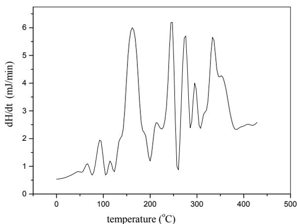
Fig. 6 - DSC curve of the aqPUR 2 sample, with the catalyst MnCAT, (2 % relating to the coating hardness)
