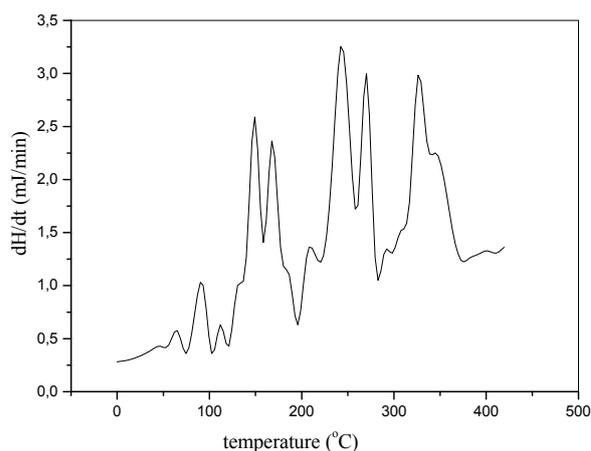
Fig. 2 - DSC curve of the aqPUR 1 sample, with the catalyst ZrCAT, (2 % relating to the coating hardness)
