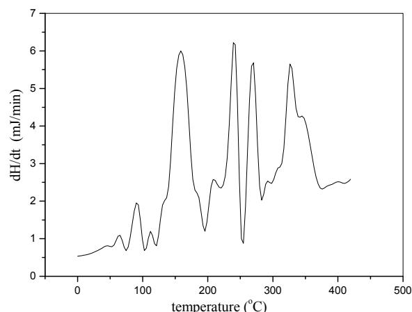
Fig. 3 - DSC curve of the aqPUR 1 sample, with the catalyst MnCAT, (2 % relating to the coating hardness)
