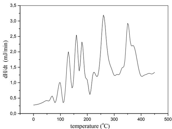
Fig. 4 - DSC curve of the aqPUR 2 simple, no catalyst
