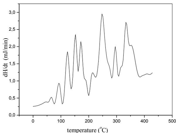
Fig. 5 - DSC curve of the aqPUR 2 simple, with the catalyst ZrCAT, (2 % relating to the coating hardness)
