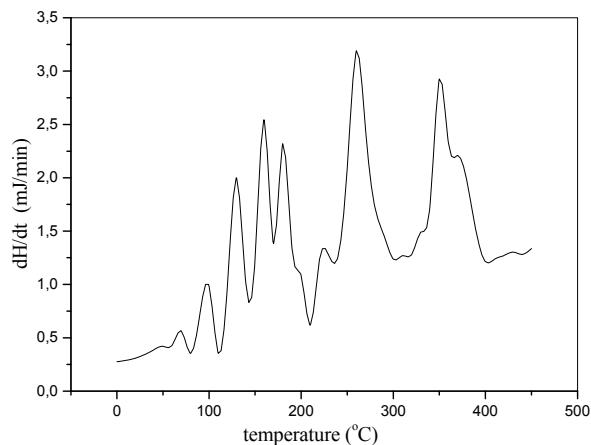
Fig. 4 - DSC curve of the aqPUR 2 sample, no catalyst
