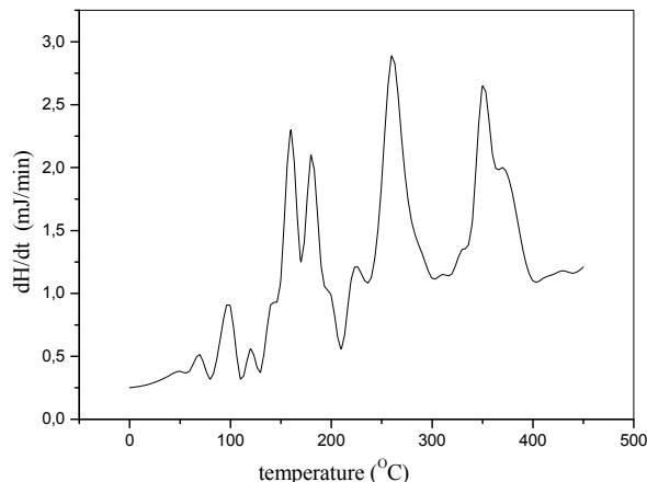
Fig. 1 - DSC curve of the aqPUR 1 sample, no catalyst
