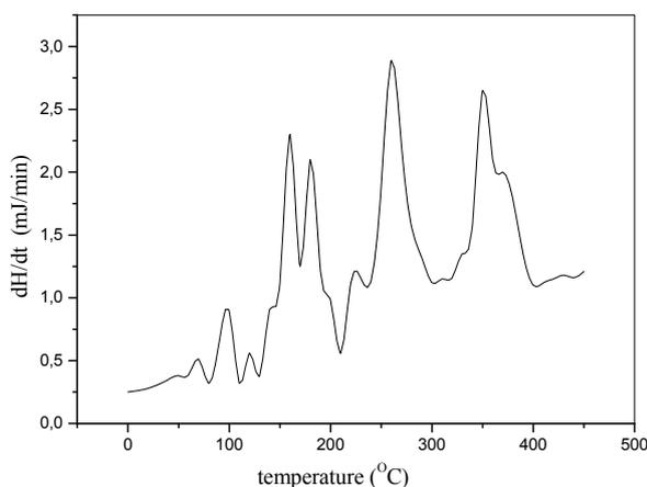
Fig. 1 - DSC curve of the aqPUR 1 simple, no catalyst
