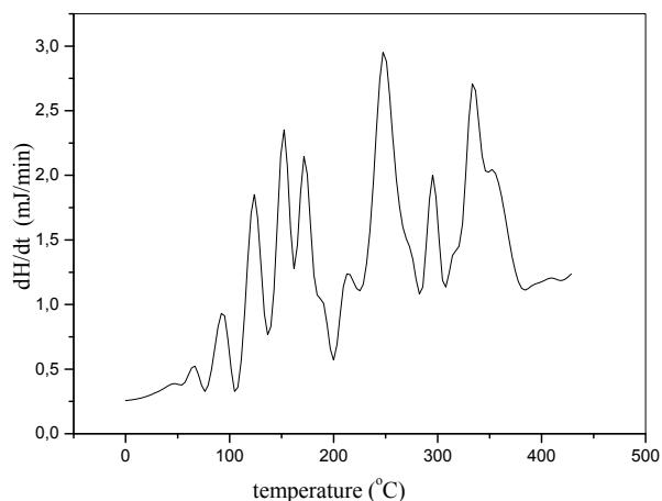
Fig. 5 - DSC curve of the aqPUR 2 sample, with the catalyst ZrCAT, (2 % relating to the coating hardness)
