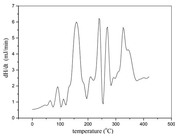
Fig. 3 - DSC curve of the aqPUR 1 sample, with the catalyst MnCAT, (2 % relating to the coating hardness)
